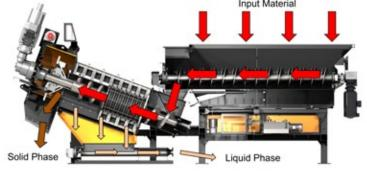
Cross Section of Doppstadt Screw Press with Feeding Hopper
