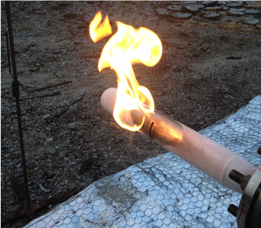
Figure 3.5. A 2" pipe without braid. A 5 by 45 mm slot is cut crosswise. The photo is taken after the test when gas still remained in the pipe.
