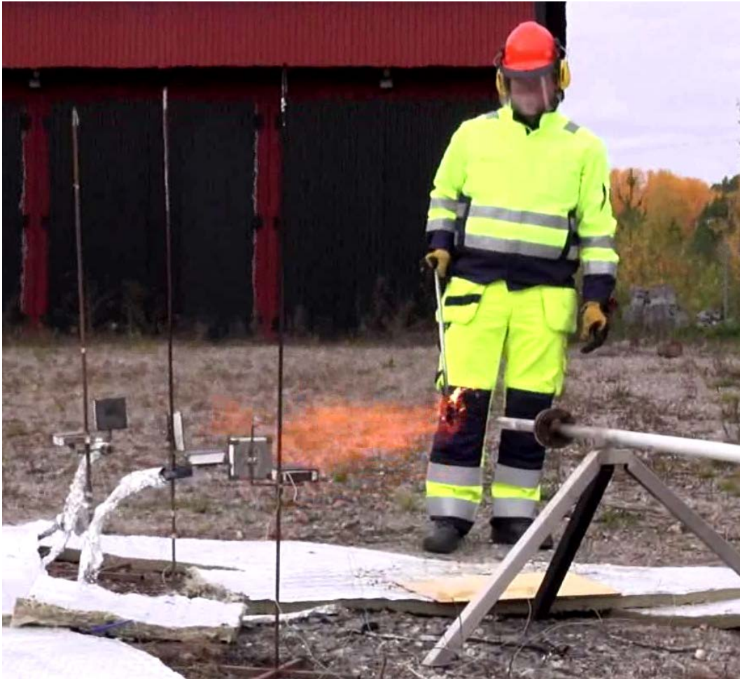
Figure 4.13. The pilot aided flame from test 3b (1" pipe with 1 mm 2 hole, no braid). The flame was never self-sustained without the presence of the pilot.
