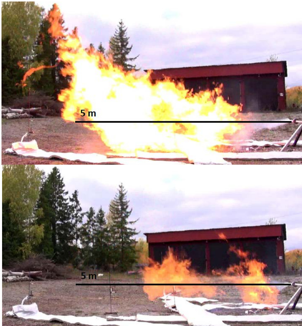
Figure 4.8. Photos from test 2b (1" pipe with 1x10 mm slot, no braid). Upper photo: a large flame pulse from the first part of the test with a pressure close to 12 bar. Lower photo: Typical behaviour for the main part of the test, with a lower pressure in the pipe (around 8 bar).
