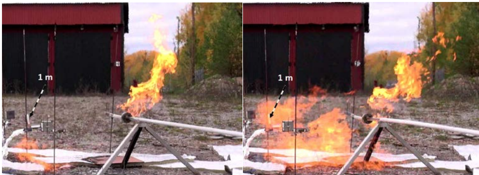
Figure 4.20. Photos from test 5 (1" hose with 1x5 mm slot, covered by a braid).
