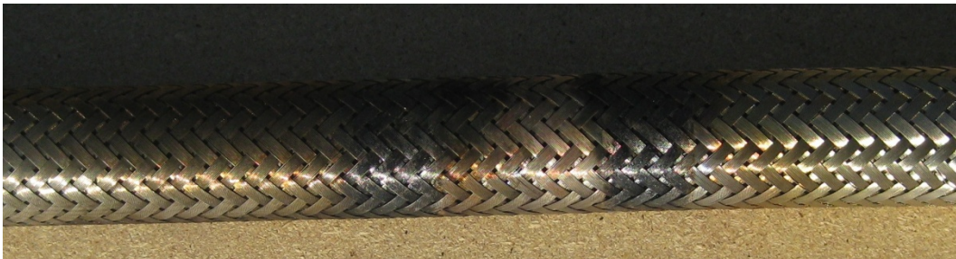
The 1" hose of test 6 (1 mm 2 hole) after the test with the braid taken still on.
