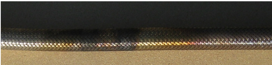
The 1" hose of test 5 (cut 5 mm) after the test with the braid still on.
