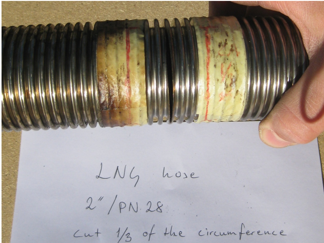
The 2" hose of test 7 after the test with the braid taken off. Note that the slot is still 1/3 of the circumference.
