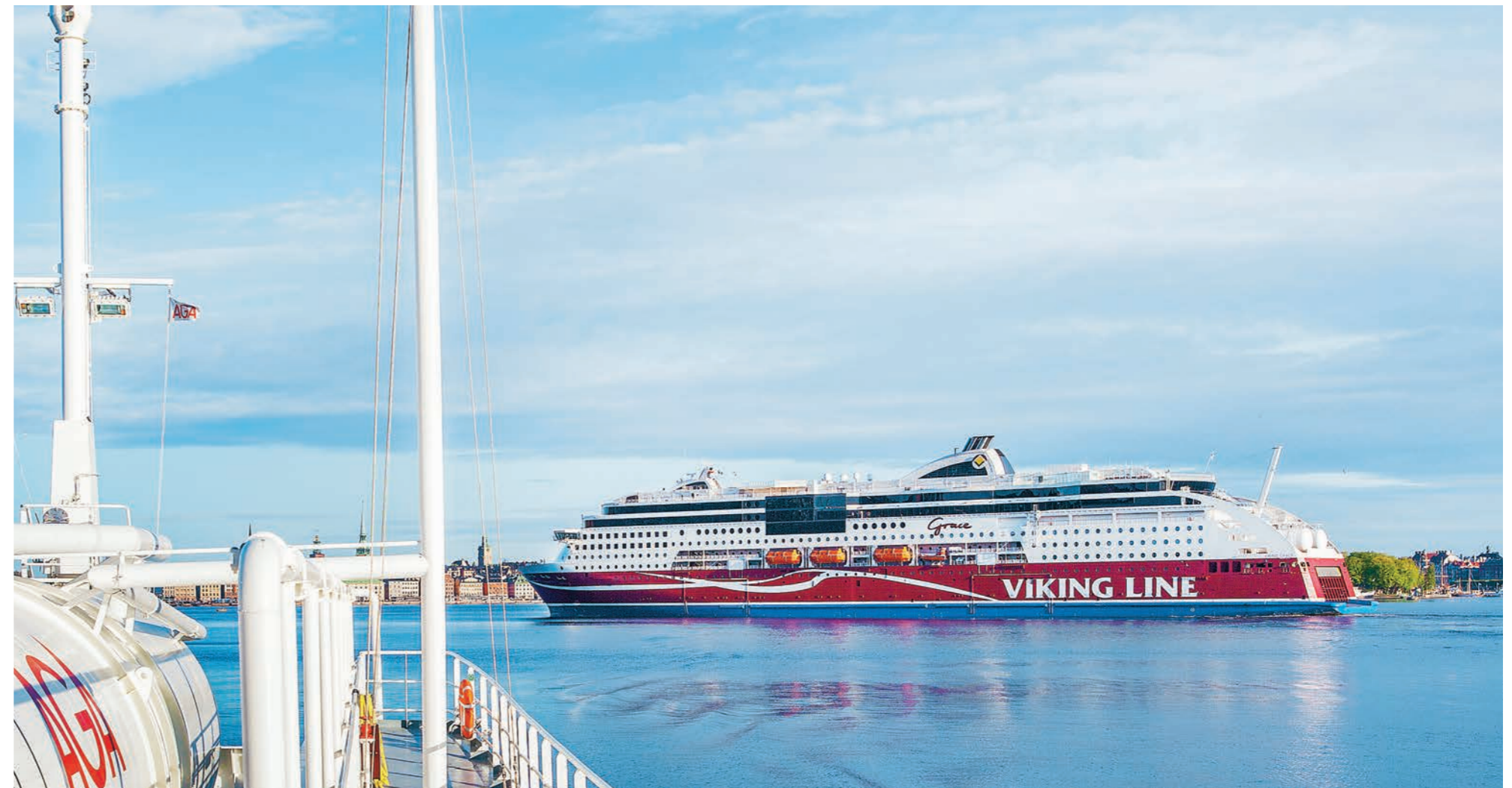
A number of Swedish and foreign shipping companies have ordered ships powered by liquefied natural gas. Viking Grace is the world's largest LNG powered passenger ferry.
